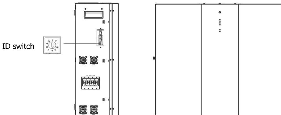
ID Switch indicates the unique ID code for each battery module. It's required to assign an identical ID to each battery module for normal operation. We can set up the ID code for each battery module by rotating the PIN number on the ID switch. From number 0 to 9, the number can be random; no particular order. Maximum 10 battery modules can be operated in parallel.
