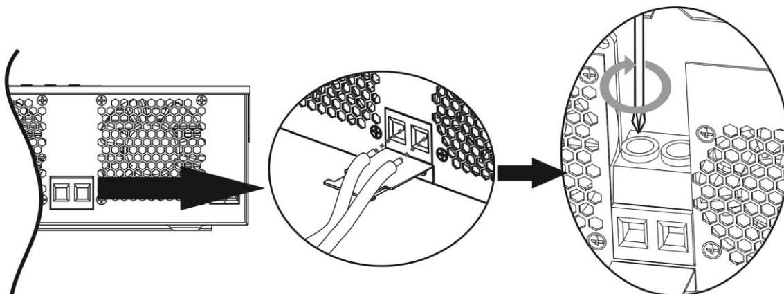
For 3K-24V model, secure assembled ring terminals to the battery terminal block with the bolts properly tightened. Refer to battery cable size for torque value. Make sure polarity at both the battery and the inverter is correctly connected and ring terminals are secured to the battery terminals.
