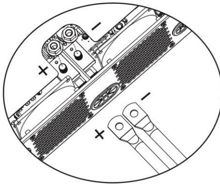
5. This step is only for 1.2KVA/2.5KVA/3KVA-48V/5KVA models. To firmly secure wire connection, you may fix the wires to strain relief with cable tie.
