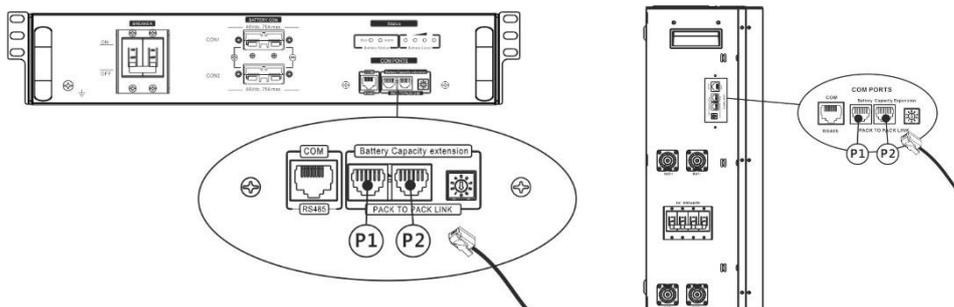
Step 2: Use supplied RJ45 cable (from battery module package) to connect inverter and Lithium battery.
