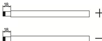
For 3KVA-24V model, refer to recommended battery spec table to purchase separately two ring terminals and battery wires. Assemble two ring terminals with battery wires based on recommended battery cable and terminal size as grounding cable. Recommended dimensions for ring terminal is D (8.4 mm) and L (39.2 mm).
